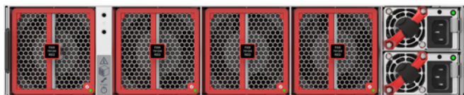
Arista 7060X5 2RU Rear View: Front to Rear airflow (red) AC Powered
